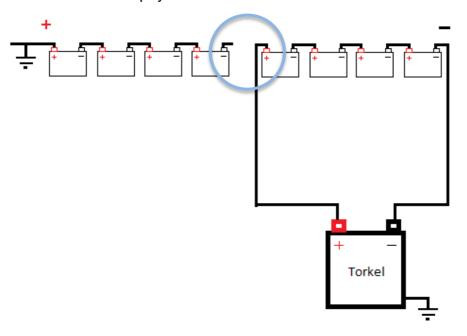
It is no problem to connect the TORKEL to the grounded section of the battery system since max allowed voltage to ground will not be exceeded. See below picture.
